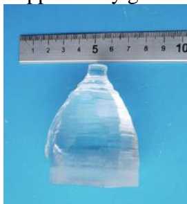
Figure 1. Typical form of \text{Li}_2\text{W}_{1-x}\text{Mo}_x\text{O}_4 crystals ( x = 0.1 ).
